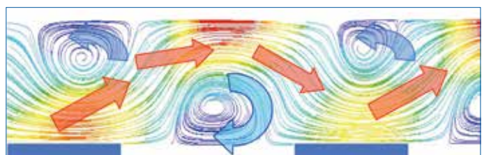
Fig. 81: Streamlines along several aeration fields
