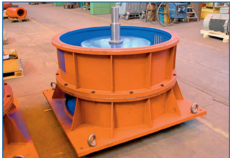
Fig. 8.1.3-b: Vertically mounted flywheel (driven by means of cardan shaft, D = 790 \text{ mm} )
