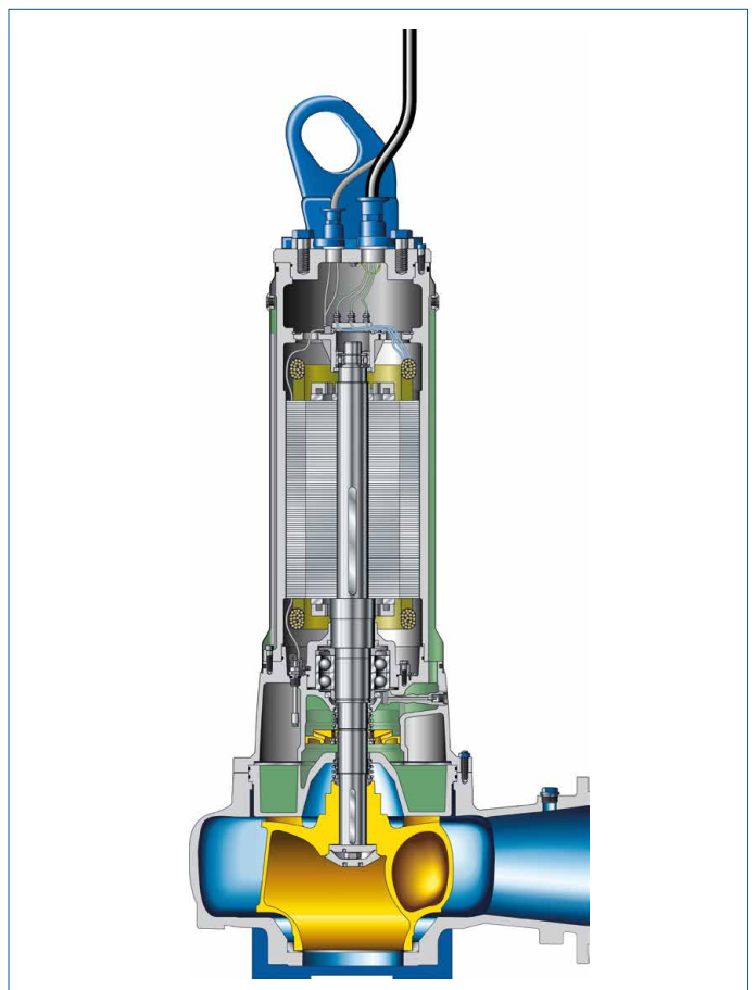
Fig. 45: Sectional drawing of a KRT > 60 kW, with cooling jacket
