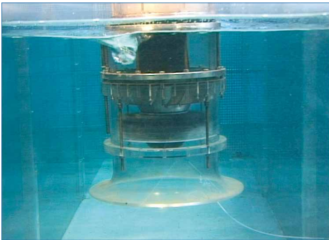
Fig. 105: Laboratory photo of a surface vortex type 3
