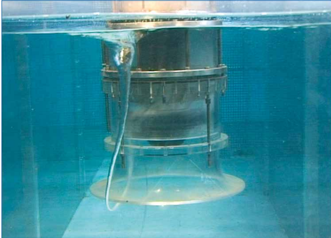
Fig. 104: Laboratory photo of a surface vortex type 6
