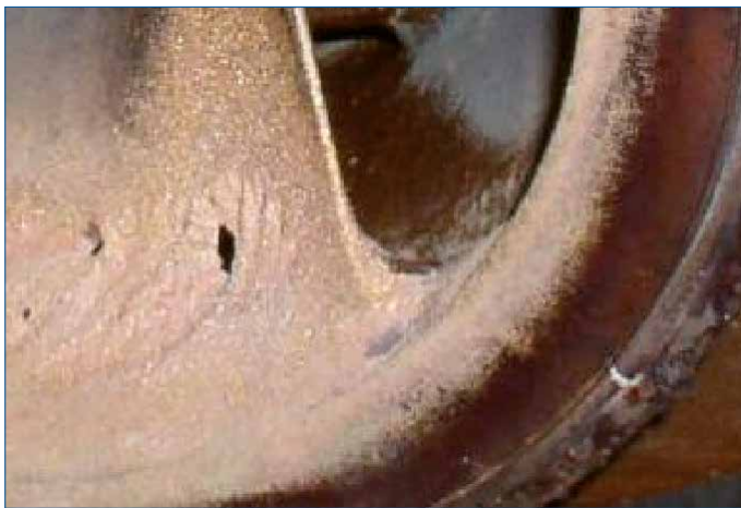
Fig. 5: Impeller showing cavitation damage (Source: KSB Centrifugal Pump Lexicon [01.06])
