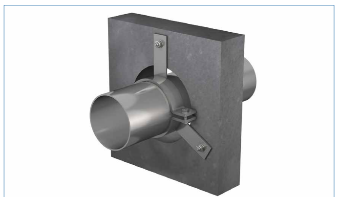
Fig. 73: Axial thrust protection as anchorage point
