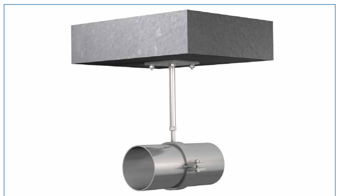
Fig. 62: Suspended from the ceiling
