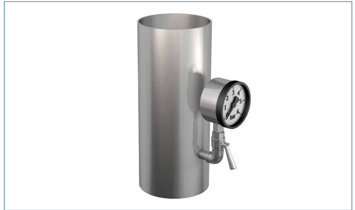
Fig. 78: Pressure measurement in vertical pipe
