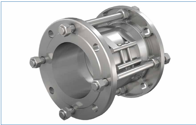
Fig. 83: Expansion and dismantling joint with axial-restraint pipe coupling and continuous threaded rods
