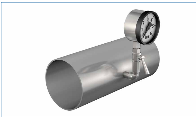
Fig. 77: Pressure measurement in horizontal pipe
