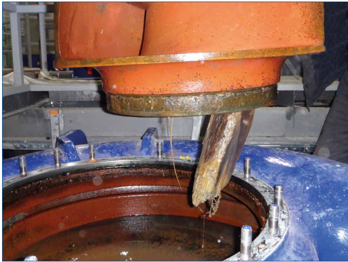
Fig. 90: Wood inside the impeller of a KRT pump
