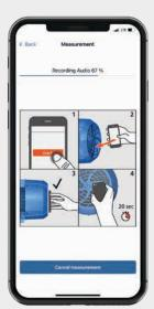
Start the measurement and hold your smartphone next to the motor. The KSB app delivers the analysis result in just 20 seconds.
