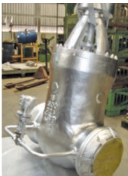
First C12A Gate & Check Valve of size 16", class 1500 manufactured successfully
