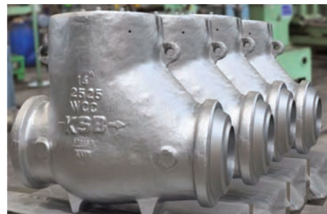
Size 14", Class 2500 High Pressure Check Valve Valve manufactured by using the existing facilities in Coimbatore Plant
