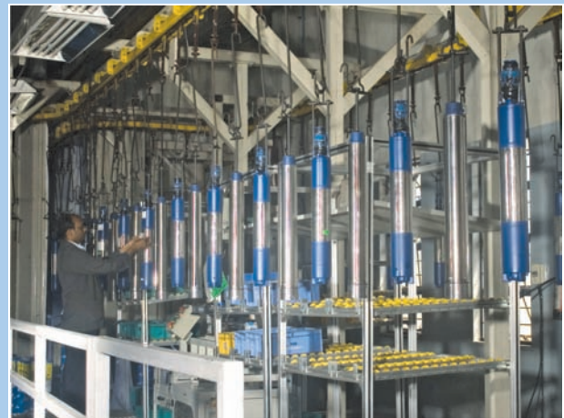
UMAI 100 motor assembly & testing automation line
