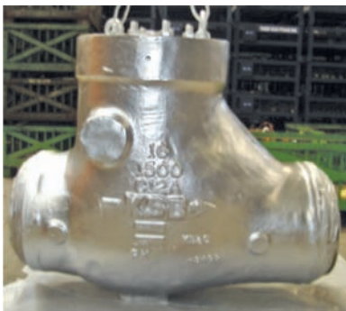
First C12A Gate & Check Valve of size 16", class 1500 manufactured successfully
