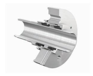
Double cartridge seal especially designed for applications with negative suction pressure. The optimised flushing channel ensures that any solids are flushed away from the inboard side of the mechanical seal.
