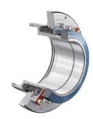
This single cartridge seal is designed specially for applications with high solids contents. Optionally, a system for periodic flushing can be connected to flush away leakage products and significantly extend the seal life.
