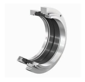
4STC is a stationary component seal for the Amarex KRT, Sewatec and Amacan pump type series. The springs are located outside the fluid handled, protected from contamination. The primary ring of the seal has been secured against falling out, making it a safer fit for vertically installed pumps.
