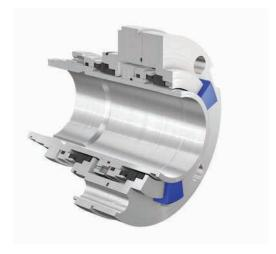
Double cartridge seal especially designed for applications with negative suction pressure. The primary ring is shrink-fitted into the metal primary ring carrier. This ensures even contact, also under fluctuating pressure and temperature conditions.
