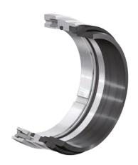
Together with the shaft protecting sleeve of the pump, the 4RD seal can be installed like a cartridge. The primary ring is shrink-fitted into the metal primary ring carrier. This ensures even contact, also under fluctuating pressure and temperature conditions.
