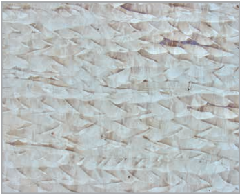
Microstructure as-built 50x
