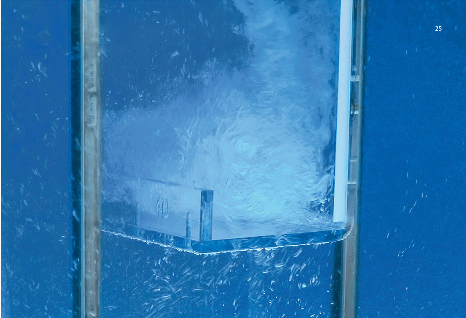
Air intake demonstrated in a model test: vortex formation with curtain wall and "balcony" 模型测试中的进气演示：在腔室内形成涡流
