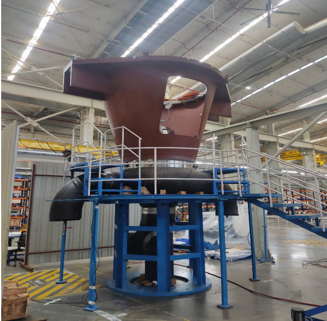
Hydro Test setup RSR 400
