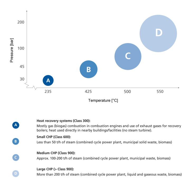
Different pressure classes (live steam) of valves for specific applications:
