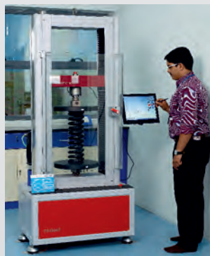
Load and deflection testing of Actuator springs
