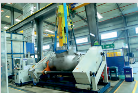
A 32 inch size valve being tested on the High pressure test bench
