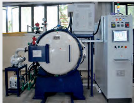
Vacuum Heat Treatment facility
