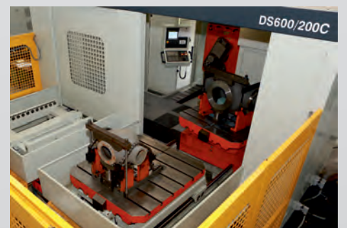
Horizontal machining centre - Valve body machining in single setting
