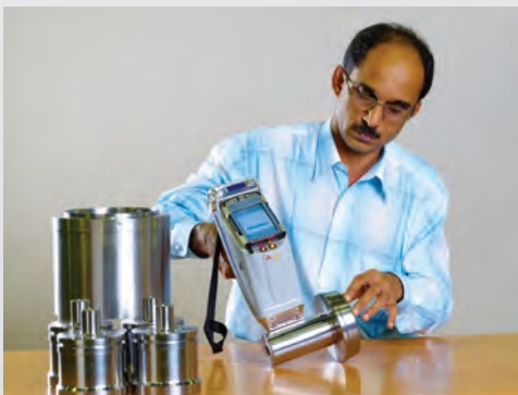
Positive Material Identification of special alloys
