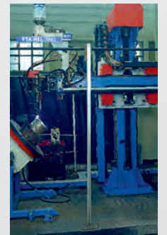
Automatic hard facing process
