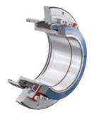
This single cartridge seal is designed specially for applications with high solids contents. Optionally, a system for periodic flushing can be connected to flush away leakage products and significantly extend the seal life.
