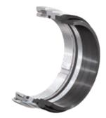
Together with the shaft protecting sleeve of the pump, the 4RD seal can be installed like a cartridge. The primary ring is shrink-fitted into the metal primary ring carrier. This ensures even contact, also under fluctuating pressure and temperature conditions.
