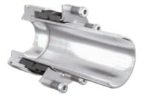
This single mechanical seal is tailored to the seal installation space of the pump. Its large external springs are insensitive to contamination and provide uniform surface pressure across the contact faces, thus ensuring a long service life. Optionally, this seal is available as a 4KD double seal.
