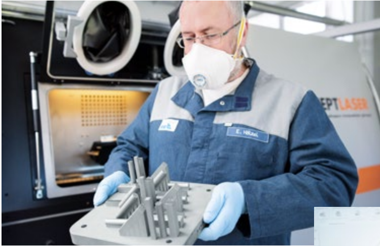
Ewald Hölzel takes away components that the production team has manufactured using the selective laser melting process.
