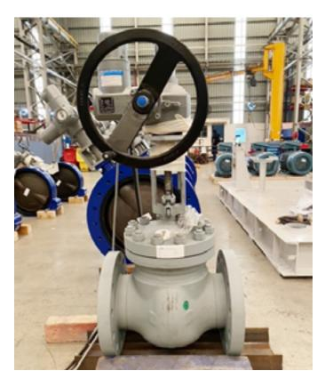
interface made of wear and corrosion resistant 17 % chrome steel or Stellite. Also, our NORI globe valve to DIN/EN with flanged, butt weld or socket weld ends, gland packing, throttling plug, non-rotating stem, bayonet-type body/yoke connection, integrated position indicator, seat/disc interface made of Stellite with Max. allowed fluid temperature: 580 °C.
