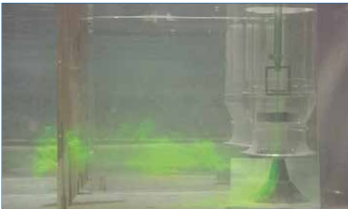
Fig. 5: Model test to observe the flow in the intake of an SEZ pump
