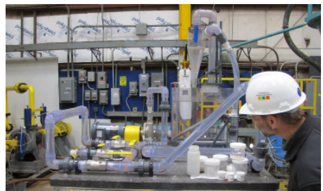
Lab demonstrations include a miniature, see-thru slurry system and full sized pipeline tests of settling and non-settling slurries.
