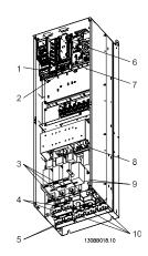
Illustration 5.26: Compact IP 00 (Chassis) with disconnect, fuse and RFI filter, frame size D4
