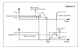
After a time delay, the relay for the fixed speed pump cuts in (staged) and this pump becomes the new lead pump. The new lead pump ramps up to maximum speed and then down to minimum speed. When ramping down and reaching the staging frequency, the old lead pump is now cut in (staged) on the mains as the new fixed speed pump.
