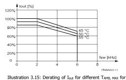
Illustration 3.15: Defailing of lout for different TAMB, MAX for enclosure E at 480 V, using 60 AVM in Normal torque mode (110% over torque)
