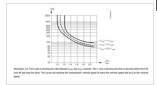
It is clear that at lower speed the ETR cuts of at lower heat due to less cooling of the motor. In that way the motor are protected from being over heated even at low speed. The ETR feature is calculating the motor temperature based on actual current and speed. The calculated temperature is visible as a read out parameter in par. 16-18 *Motor Thermal* in the frequency converter.
