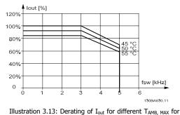
Illustration 3.13: Derating of I<sub>out</sub> for different I<sub>AMB, MAX</sub> for enclosure D at 690 V, using 60 AVM in Normal torque mode (110% over torque). Note: P400 *only*.
