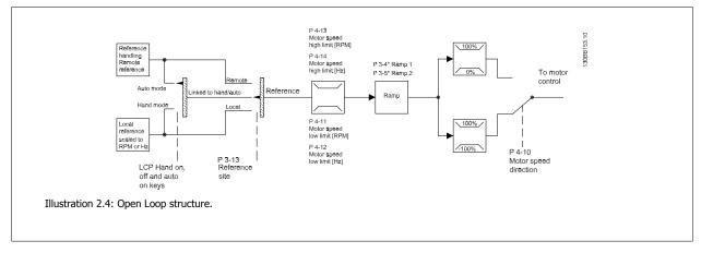
In the configuration shown in the illustration above, *par. 1-00 Configuration Mode* is set to Open loop [0]. The resulting reference from the reference handling system or the local reference is received and fed through the ramp limitation and speed limitation before being sent to the motor control. The output from the motor control is then limited by the maximum frequency limit.
