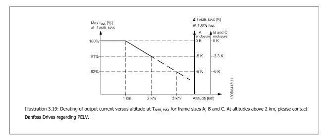
An alternative is to lower the ambient temperature at high altitudes and thereby ensure 100% output current at high altitudes. As an example of how to read the graph, the situation at 2 km is elaborated. At a temperature of 45° C (T<sub>AMB, MAX</sub> - 3.3 K), 91% of the rated output current is available. At a temperature of 41.7° C, 100% of the rated output current is available.
