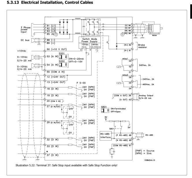
Very long control cables and analog signals may in rare cases and depending on installation result in 50/60 Hz earth loops due to noise from mains supply cables.
