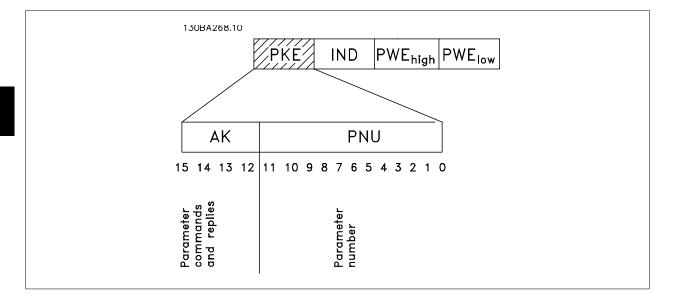
Bits no. 12-15 transfer parameter commands from master to slave and return processed slave responses to the master.
