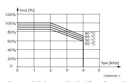
Illustration 3.12: Derating of  $I_{out}$  for different  $T_{AMB, MAX}$  for enclosure D at 690 V, using SFAVM in Normal torque mode (110% over torque). Note: *not* valid for P400.
