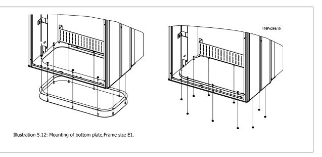
The bottom plate of the E1 frame can be mounted from either in- or outside of the enclosure, allowing flexibility in the installation process, i.e. if mounted from the bottom the glands and cables can be mounted before the frequency converter is placed on the pedestal.
