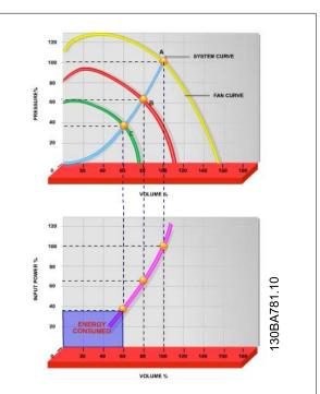
Illustration 2.2: When using a frequency converter to reduce fan capacity to 60% - more than 50% energy savings may be obtained in typical applications.
