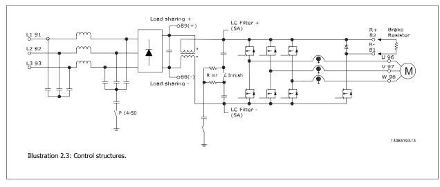
The frequency converter is a high performance unit for demanding applications. It can handle various kinds of motor control principles such as U/f special motor mode and VVC plus and can handle normal squirrel cage asynchronous motors. Short circuit behavior on this FC depends on the 3 current transducers in the motor phases.
