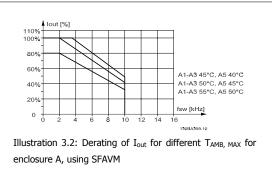
In enclosure A, the length of the motor cable has a relatively high impact on the recommended derating. Therefore, the recommended derating for an application with max. 10 m motor cable is also shown.
