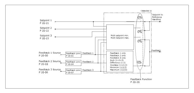
Feedback handling can be configured to work with applications requiring advanced control, such as multiple setpoints and multiple feedbacks. Three types of control are common.
