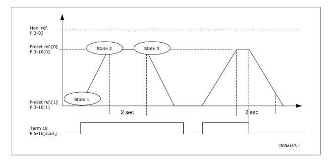
Set the ramping times in par. 3-41 Ramp 1 Ramp Up Time and par. 3-42 Ramp 1 Ramp Down Time to the wanted times
