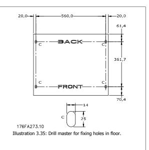
Mount the drive on the pedestal and fix it with the included bolts to the pedestal as shown on the illustration.
