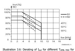
Illustration 3.6: Derating of  $I_{\text{out}}$  for different  $T_{\text{AMB},\mbox{ MAX}}$  for enclosure B, using SFAVM in Normal torque mode (110% over torque)
