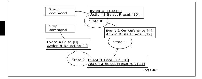
Set the Smart Logic Control in par. 13-00 SL Controller Mode to ON.
