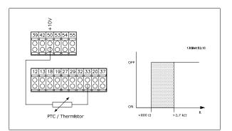
Using an analog input and 10 V as power supply:
