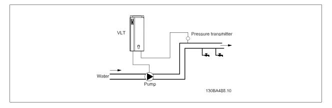
In a water distribution system, the pressure is to be maintained at a constant value. The desired pressure (setpoint) is set between 0 and 10 Bar using a 0-10 volt potentiometer or can be set by a parameter. The pressure sensor has a range of 0 to 10 Bar and uses a two-wire transmitter to provide a 4-20 mA signal. The output frequency range of the drive is 10 to 50 Hz.
