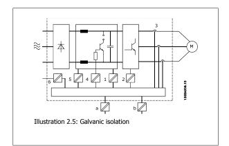
The functional galvanic isolation (a and b on drawing) is for the 24 V back-up option and for the RS 485 standard bus interface.
