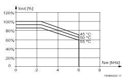
Illustration 3.11: Derating of  $I_{out}$  for different  $T_{AMB, MAX}$  for enclosure D at 690 V, using 60 AVM in Normal torque mode (110% over torque). Note: *not* valid for P400.
