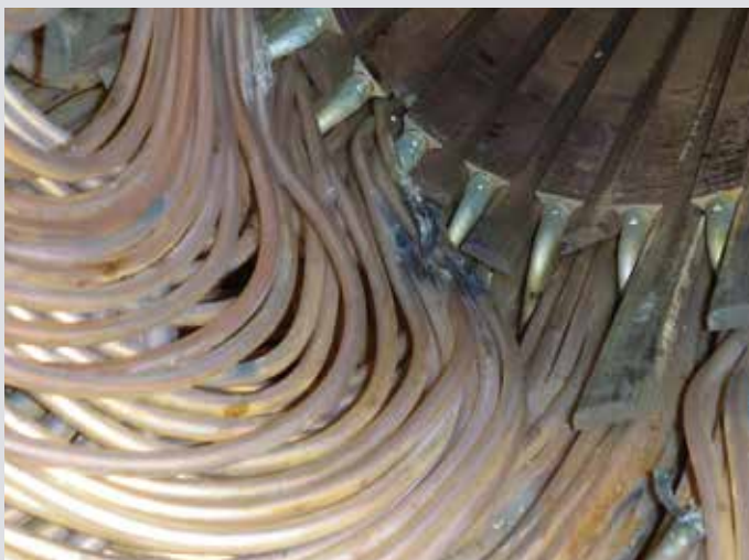
Burnt submersible motor windings
